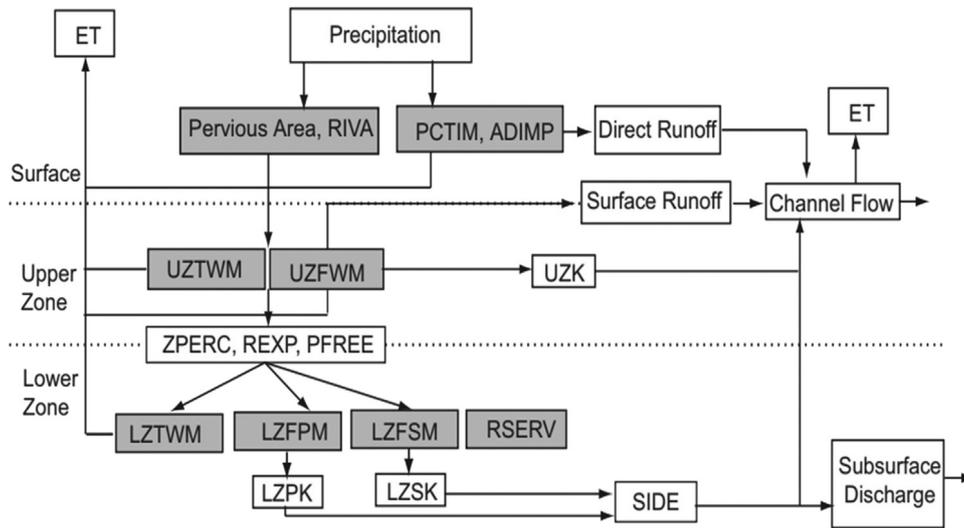
Fig. 10. A schematic of the SAC-SMA model (Tang et al., 2007).
