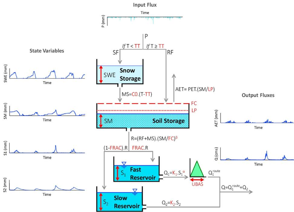
Fig. 3. System architecture of the HBV-SASK hydrologic model (Razavi and Gupta, 2019).
