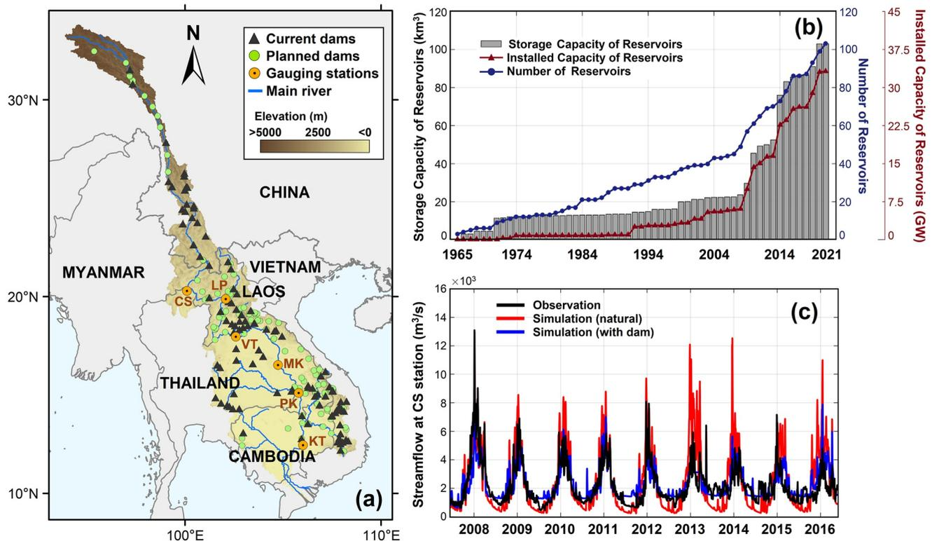
**Figure 1.** (a) The Lancang-Mekong River Basin (LMRB) with the dams and streamflow gauging stations (including Chiang Sean [CS], Luang Prabang [LP], Vientiane [VT], Mukdahan [MK], Pakse [PK], Kratie [KT]). (b) Changes in the number, installed capacity and storage capacity of reservoirs during 1965–2021 in LMRB. (c) Observed and simulated daily streamflow at CS stations in LMRB during 2008–2016 (Table S1 in Supporting Information S1).
